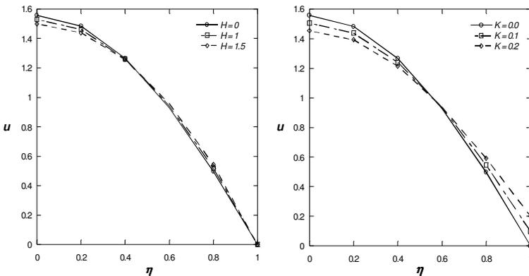
Figure 2: Axial fluid velocity profiles for different values of  $H$  and  $k$  ;  $S = 1$  and  $Re = 1$ .
