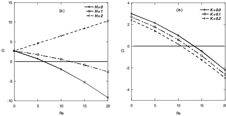
Figure 4: Wall shear stress for different values of  $H$  and  $k$ ; (a) when  $k = 0.1$  and (b) when  $H = 1$ .
