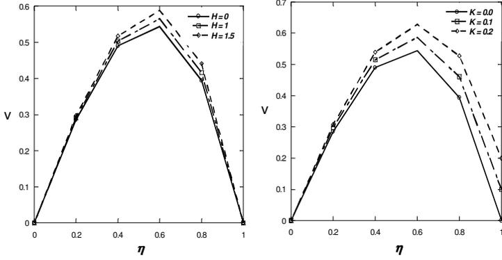
Figure 3: Normal fluid velocity profiles for different values of  $H$  and  $k$ ;  $S = 1$  and  $Re = 1$ .
