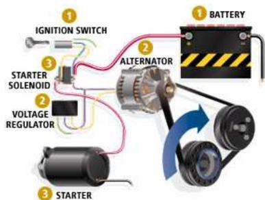
Fig: Starting and Charging system
