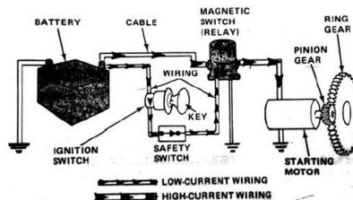
Fig: Schematic diagram of starting system
