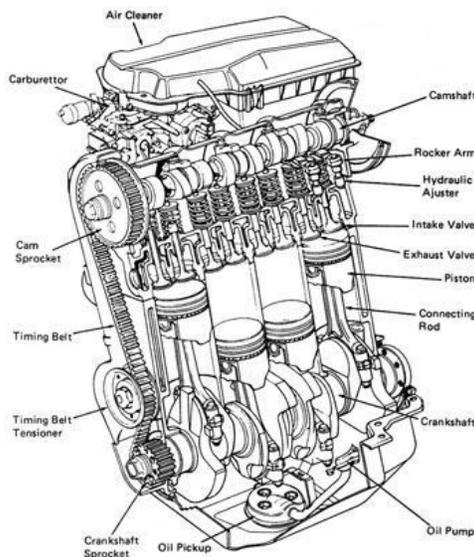
Fig: Cutaway view of a IC engine showing important parts
