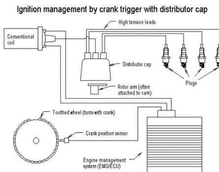
Fig: Electronic ignition system
