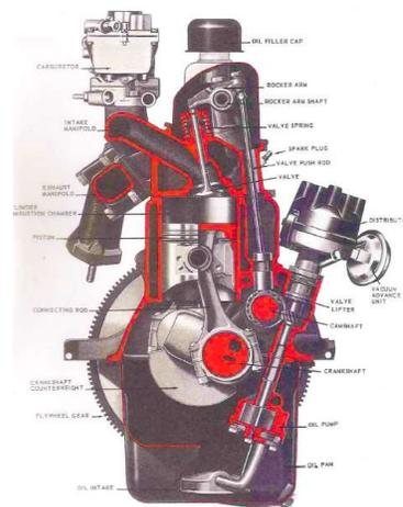
Front section view, Ford Falcon, 144 cu. in., 6-cylinder engine, with principal parts identified.
