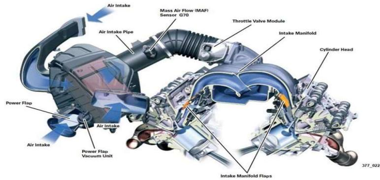
Fig: Air intake system of Audi vehicle
