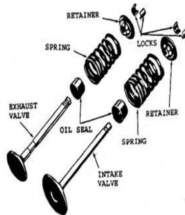
Fig: Intake and Exhaust valve with important parts
