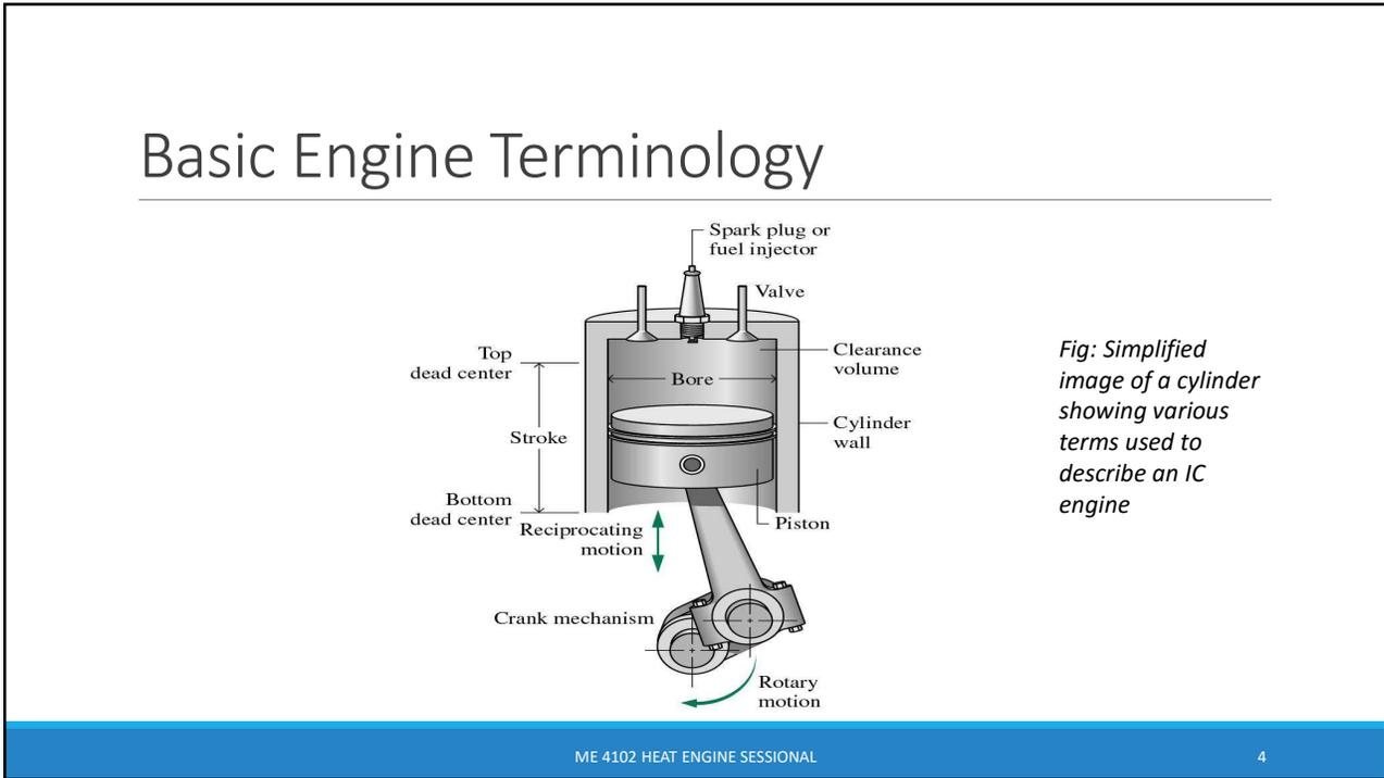
1. **Bore:** The nominal inside diameter of the engine cylinder is called bore.
