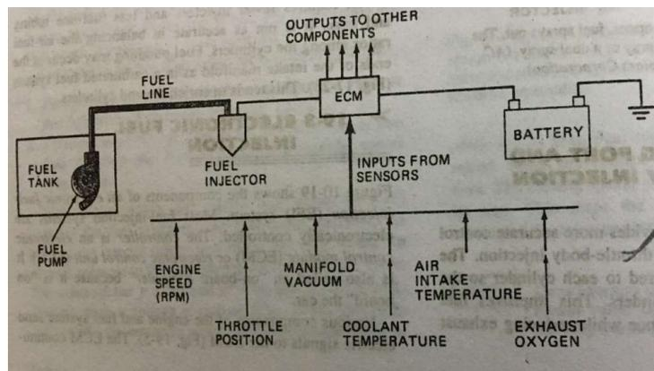
**Fig: Simplified electronic fuel-injection system.**
