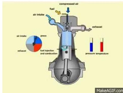
Same as that of four stroke SI engine but at the compression stroke air fuel mixture ignites by self ignition of the diesel fuel. In Diesel engines when the air is compressed to such a large extent it's temperature rises well above 600 degree Celsius. This temperature is above the **self ignition temperature** of diesel fuel which when injected into the compressed air explodes to create the power to drive the crankshaft.
