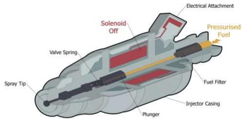
Fig: EFI cutaway model
