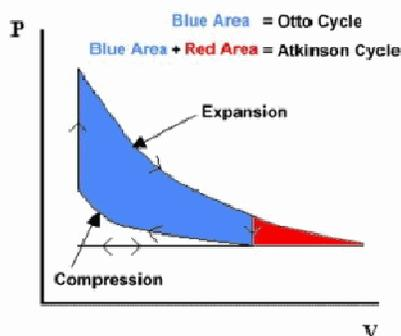
Fig: P-V diagram of Atkinson cycle
