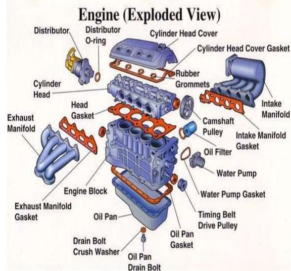
Fig: Exploded view of a IC engine
