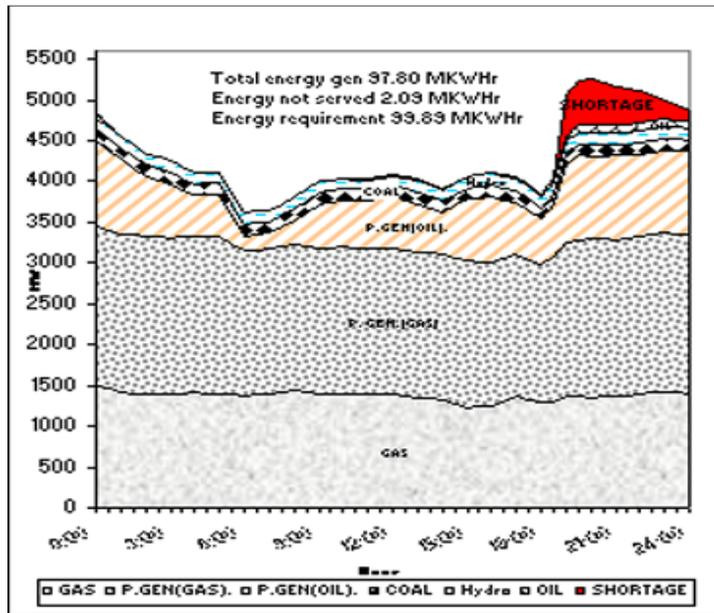
Fig. 5 Energy curve of a typical day from the month of June to October
