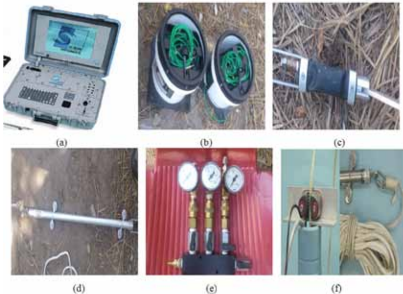
Figure 2 Different components of Suspension PS Logging Test Equipment used in this study.
