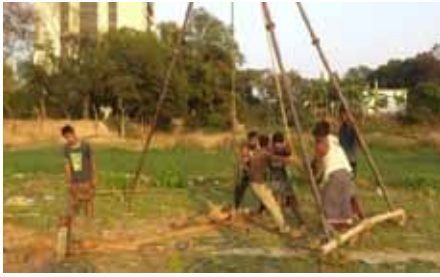
Figure 3 SPT Test at MIST
